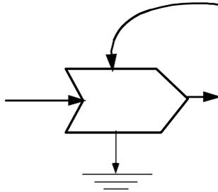
**CONSTANT GAIN AMPLIFIER**-- A special interaction symbol is used if the output is controlled by one input (entering symbol from left), but most of the energy is drawn from the other (entering from the top).
